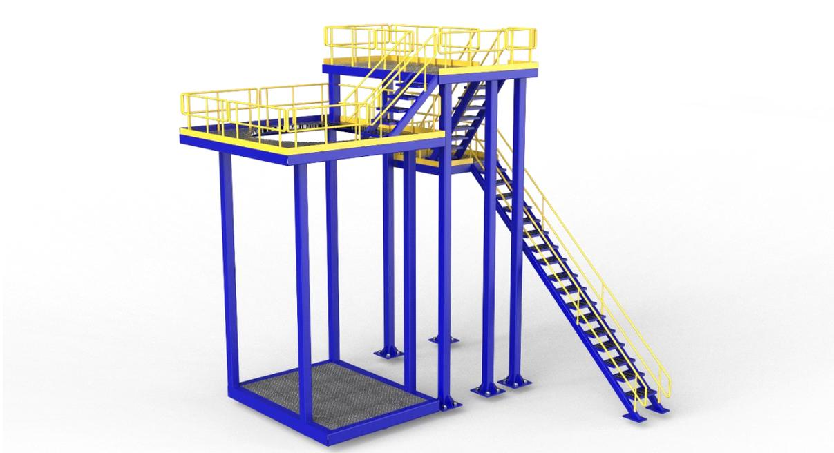
The platform structure of a VI (Viscosity Index) improver plant serves as a crucial support system for various equipment, machinery, and personnel involved in the manufacturing process. It provides a safe and accessible working environment, allowing for efficient operation, maintenance, and monitoring of the plant's operations. These platforms are strategically located within the plant to provide access to key areas and equipment while optimizing floor space utilization.
