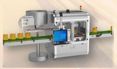
brought out through chute and supported at the end by spring loaded fingers the containers as it comes out of the filling station moves to the capping unit, where-in it picks up the cap and goes towards the capping head. The caps are subsequently tightened through magnetic clutch system. The capped bottles finally emerge out of the machine through discharge conveyor. The speed can be adjusted through the VFD on
