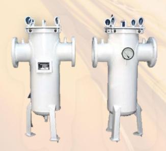
Unfiltered liquid enters the strainer housing and passes down them. Solids are retained inside of strainer mesh which is removed when the unit is serviced. strainers are normally supplied with a spring arrangement at the top of the filter element.
