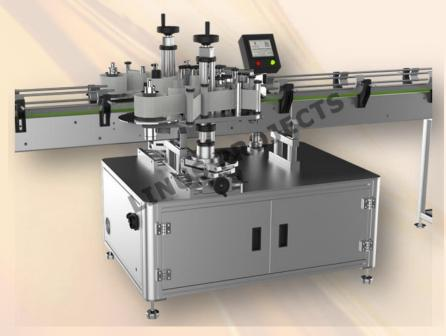
The Automatic Self-Adhesive Sticker Labelling Machine is one of the most users friendly. The machine is used for two sides labelling on the flat surfaces of different sizes of flat containers. It is capable of labelling up to 40 containers per minute depending on products and label size. The automatic model is equipped with a belt spacing device resulting in a simple "No change parts required". The flat containers are positioned & curate spacing
