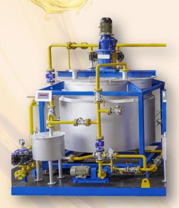
One of the key features of the skid-mounted lube oil blending plant is its versatility. The system accommodates a wide range of base oils and additives, allowing for the formulation of a diverse array of lubricant products tailored to specific industry needs. The modular design ensures flexibility in production, enabling manufacturers to adapt quickly to changing market demands and product specifications.
