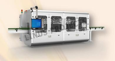
It is volumetric type complete with a 50 Ltrs stainless steel storage hopper. The pump is suitable for filling of coolants in plastic containers from 250ml to 5 Ltrs. A 1 HP electric motor drives the pump. An electronic control panel with volume control setting is provided. The Bottles are to be placed manually on Machine. the nozzles dive into the Bottles and filling take place. The volume adjustment is manual through cam adjustment. The
