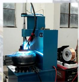
Other parts such as foot ring, backing strip, top ring and turned components are manufactured separately. Now both the halves are joined with a backing strip prior to their welding. After welding complete cylinder undergo stress relieving normalizing process in suitable heat treatment furnaces. After stress relieving sand blasting is done.
