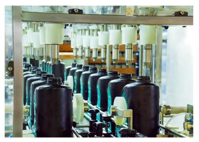
Linus Projects (INDIA) machines for the Lube oil and Grease industry, one of the leading Indian manufacturers of filling and automatic filling machines like as a filling, capping, and labelling line guides, organizes, fills, and then releases bottles in an automatic bottle packaging line.
