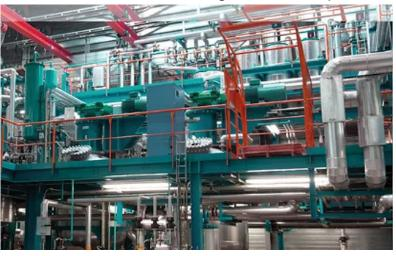
temperature control and minimizing heat transfer to the uncovered vessel wall, thereby ensuring superior quality for your lubricants. To reduce contamination within the blending vessel, a conical bottom and an efficient spray nozzle system are utilized to thoroughly flush the vessel after each batch blending.
