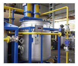
Blender is provided with an additive dozing bunker. Drive consists of electric motor coupled to a heavyduty gearbox by couplings. Output shaft of the gearbox is coupled to stool housing complete with oil seals, gland bearings, and packing's. The blending vessel can withstand a temperature of 200°C. It is duly insulated with rock wool and cladded with GI sheets.
